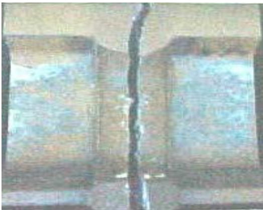
FIG. 50 : 411 - WELDING, FLASH BUTT JOINT, TRANSVERSE CRACK
