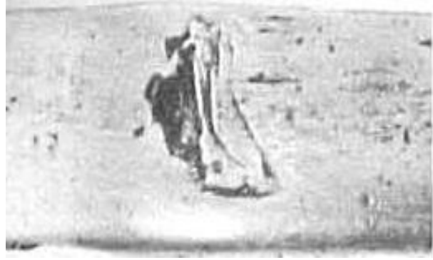
FIG. 39 : 2251 - HEAD, SURFACE, WHEEL BURN ISOLATED
