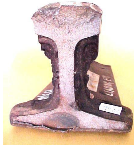
FIG. 51 : 421 - WELDING, THERMIT JOINT TRANSVERSE CRACK
