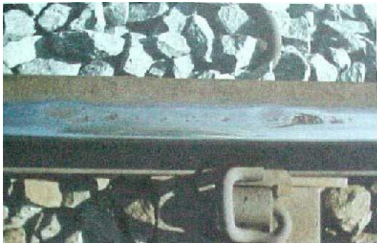
FIG. 40 : 2252 - HEAD SURFACE, WHEEL BURN REPEATED
