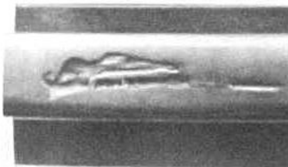
FIG. 36 : 1211 OR 2211 - HEAD, SURFACE, SHALLOW SURFACE DEFECT (FLAKING)
